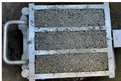
Fig. 71: Filled formwork
