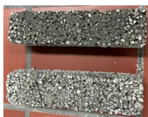
Fig. 78: Left: specimen dried in oven; right: specimen dried at room temperature
