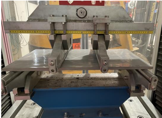
Fig. 45: Flexural strength test
