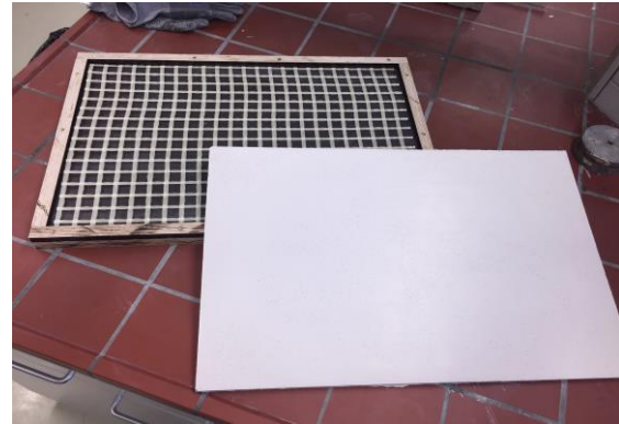
Fig. 46: Plates with glass textile in the middle of the place
