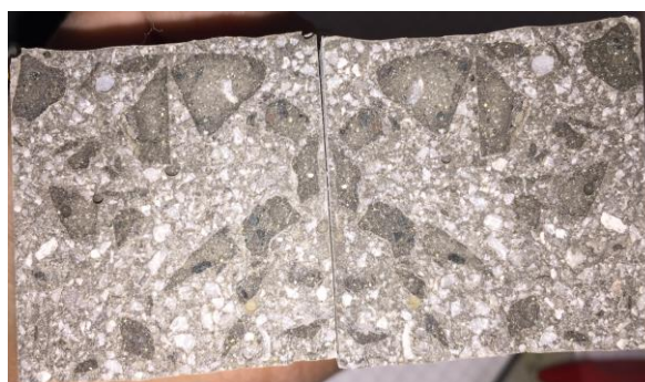
Fig. 61: UHPC used as RCA in Normal Strength Concrete mixes
