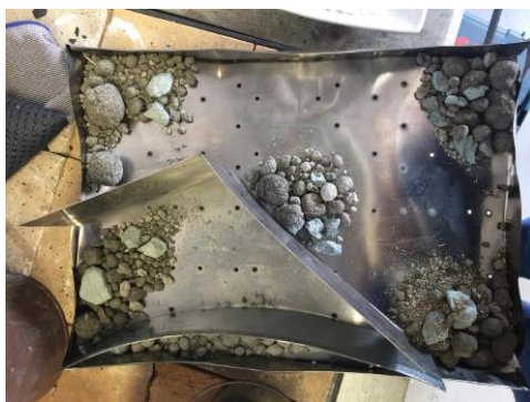
Fig. 65: Balls before firing
