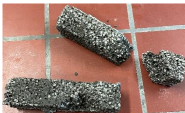
Fig. 76: Samples stuck to formwork
