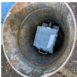
Fig. 74: Glass plate as protection for the test specimens
