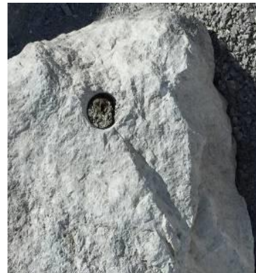
Fig. 23: Perforation hole made by drilling machine
